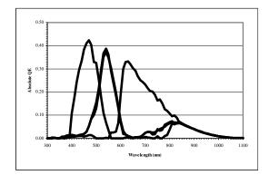
Figure 1. Absolute quantum efficiency Kodak KAI-11000CM image sensor.
