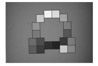
Figure 3. OECF Test Target.
