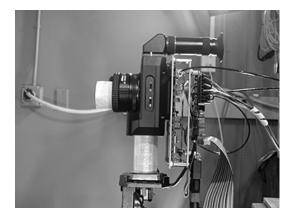
Figure 2. Horseman Digiflex Camera and The KODAK KAI-11000CM Image Sensor System.
